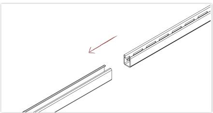
Put the profiles on the ground and slide the vertical wall profiles in the c-profiles. Because of the fact that the upper and lower screw holes each have a distance from 2 cm to the end of the profile, that means they are the same at the top and the bottom, it is not necessary to consider the direction of the vertical wall profile while mounting it.
