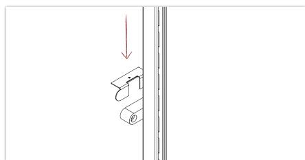
To align the shelf in height, turn the adjustable feet downward as far in or out until the foot is flush with the c-profile below. Then also the vertical wall profile is in the same line with c-profile at the top. After hanging the first shelf row, it is recommended to check the horizontal line with an air level on the shelves and make any necessary adjustments.
