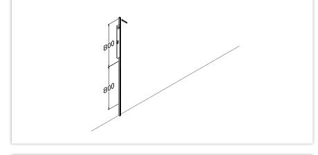
Turn the vertical wall profile by 90° in the horizontal line and align it with an air level. Now mark the second profile, depending on the used grid at a distance of 80 or 120 cm from the marks you created earlier. Repeat this for all three positions of the wall holders and for all profiles used.
