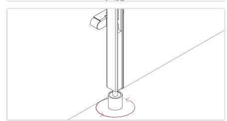
The bottom supports can be frontal set in the profile by the supplied magnetic tool, they have to be rotated by 90° and are therefore safe in the hidden gridding of the profile. All elements that are provided for the vertical wall profile can be mounted in that they enter the top or the bottom of the profile. Their sides do have hooks at the rear upper end which rest on the bottom supports. Webs on the lower rear end retain the elements in the profile.
