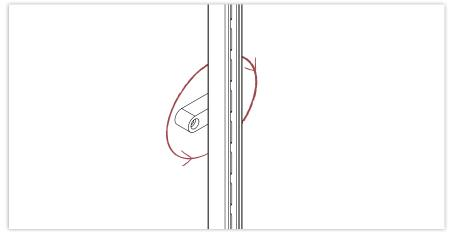
When all profiles are mounted the magnetic covers can be slid onto the wall holders to hide the screws.
