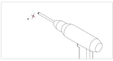
Please use the borer suitable for the used anchor bolts and bore all holes for the wall holders. Do not bore the middle mark, here is no hole needed.
