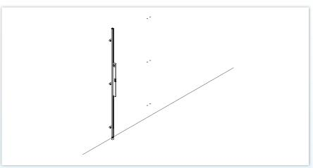
Place the profile unit of c-profile, vertical wall profile and wall holders against the wall and align it with an air level.
