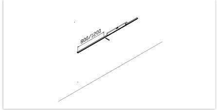
Use the wall holders as a template to mark the drill holes. You have characterized the axis of the wall holders so far but not the drill holes.
